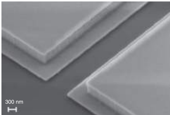
Figure 4.11 Scanning electron microscope image showing part of a Josephson array with quadruple stacks of Nb/NbSi/Nb junctions. The NbSi barriers appear dark while the niobium appears lighter. The image was taken at an intermediate step of the fabrication process and does not show all details of a complete Josephson array. Source: Courtesy of O. Kieler, PTB.
