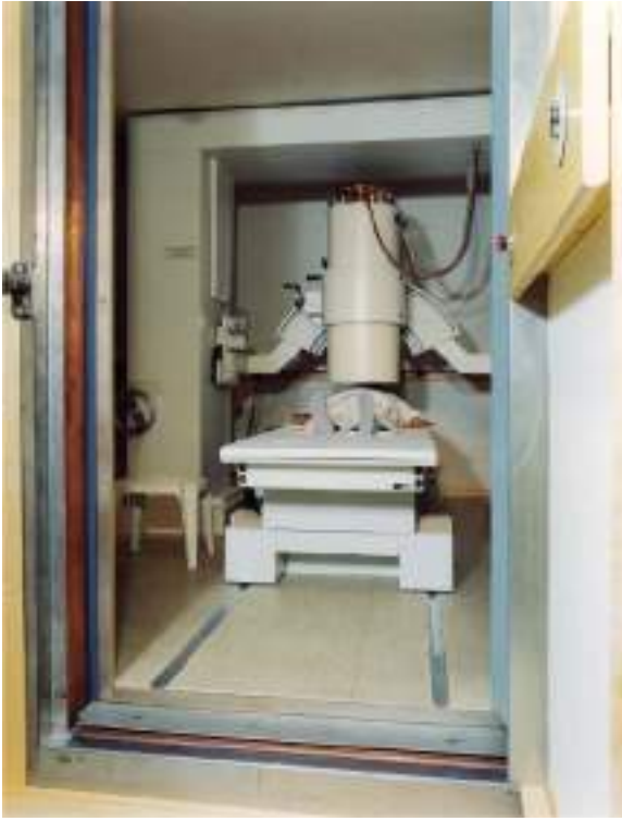
Figure 4.23 Eighty-three-channel SQUID system aligned above a patient for MCG measurements. Source: Courtesy of PTB.
