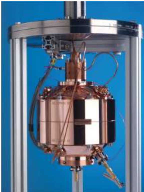
Figure 8.2 Photo of the assembled National Physics Laboratory (NPL) 1 l copper AGT resonator. Source: Reproduced with permission of NPL Management Limited.
